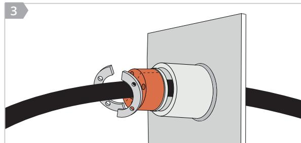
If the cable or pipe is already installed, open the SR sealing and place it over the cable or pipe.
