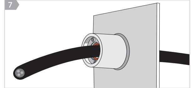
Lubricate the inner sealing surfaces and the cable or pipe using MCT Brattberg Lubricant.
